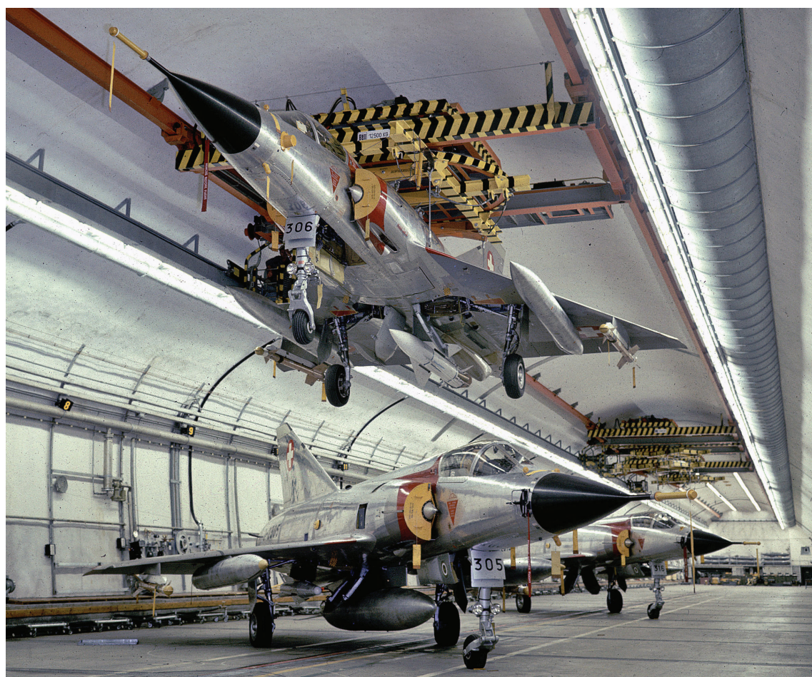
BELOW: Inside one of the secret aircraft caverns, a IIS with an AS30 missile and two Sidewinders is lifted over a sister aircraft. The radome had to be manually folded sideways for turn-around. RUAG
