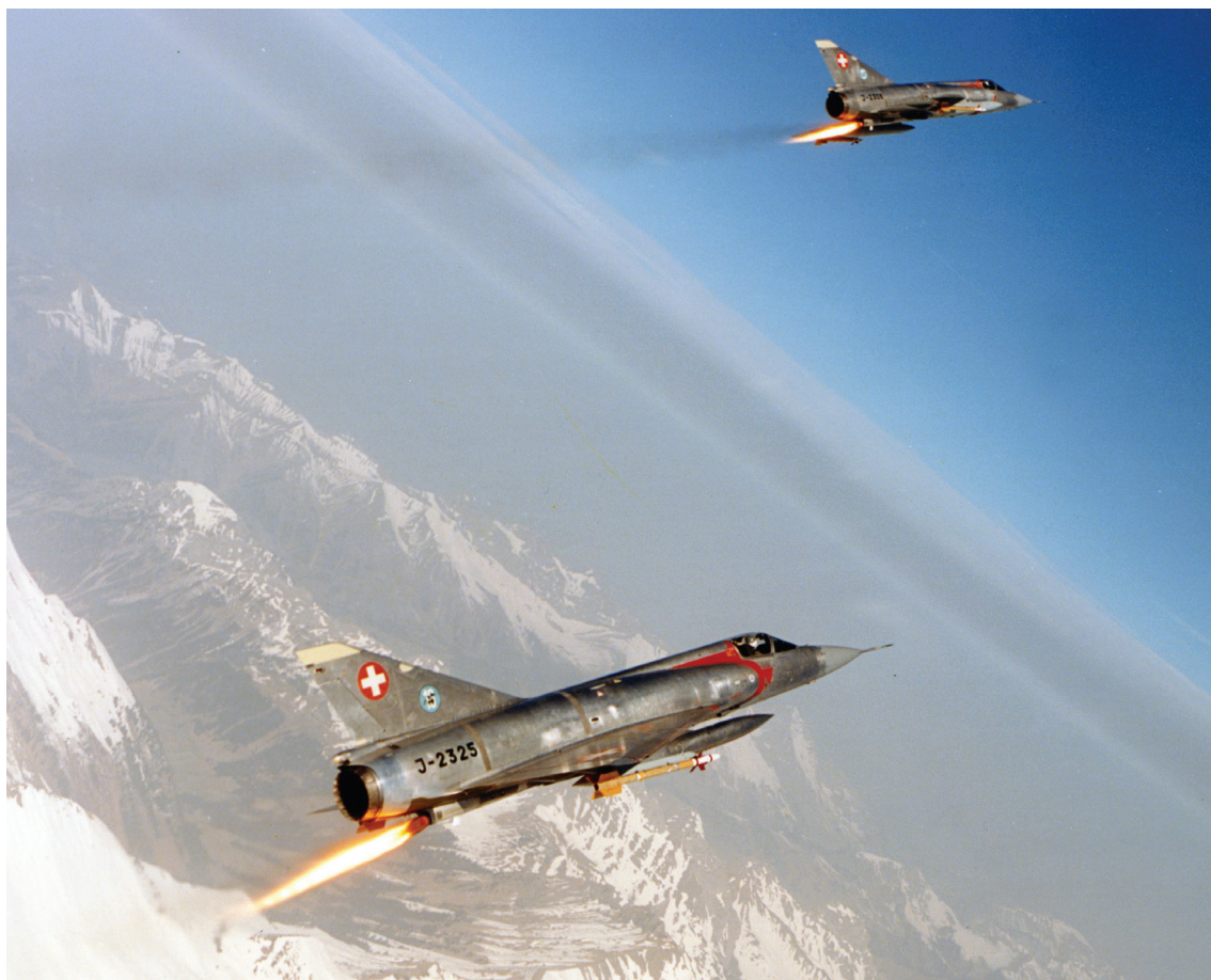
ABOVE: The SEPR rocket engine improved the Mirage III's supersonic acceleration and enabled zoom climbs up to 22,000m (72,000ft). It's demonstrated here by a pair of IIIS fighters. SWISS AIR FORCE
